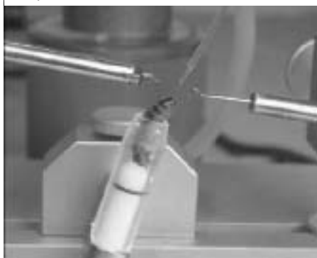
fig. 5: To more closely simulate natural mating, the queen holding tube is positioned 180° from the standard previously used. The hooks are reversed, the pressure grip forceps are on the left and the ventral hook to the right. To more closely simulate natural mating, the queen holding tube can be positioned 180° from the standard used. The hooks are reversed, the sting hook or forceps placed on the left and the ventral hook to the right, as in Fig.5. A comparison of the two positions is diagrammed in Fig. 7.
